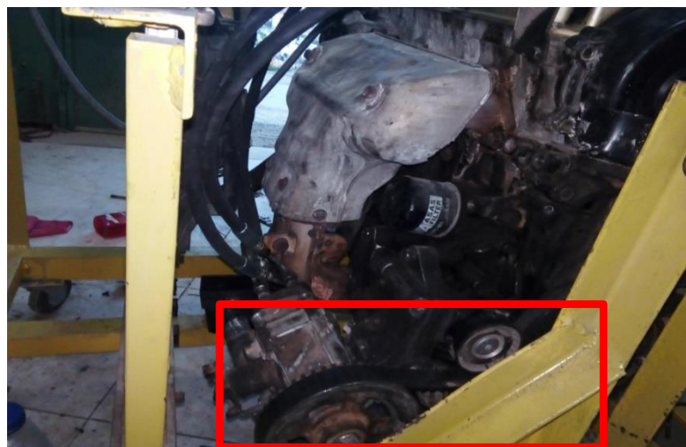
Figure(4.15): the pulley and timing belt
