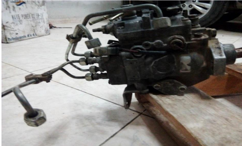
Figure (4.11): diesel distributing rotary pump with mechanical governor
