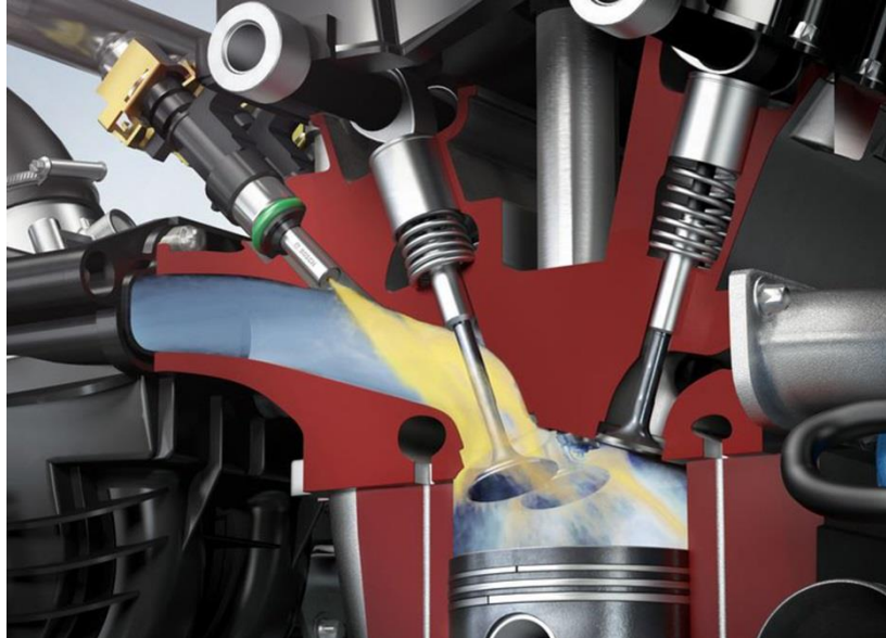
Figure (3.2): Intake manifold WIS.[12]
