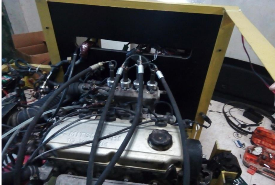
Figure (4.13): Injectors connected with pressurized water pipes
