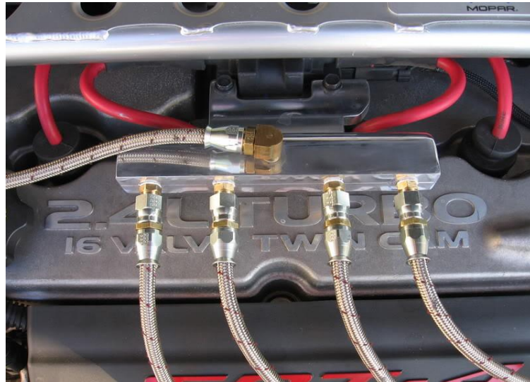
Figure (3.9): Common Rail 4-injectors [19]
