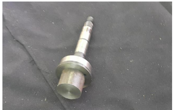
Figure (4.8): water pump construction a) compressor and diesel pump , b) shaft
